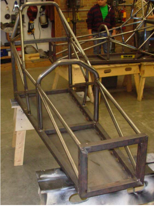
A front view of our car, which shows the welds on the top of the floor.
